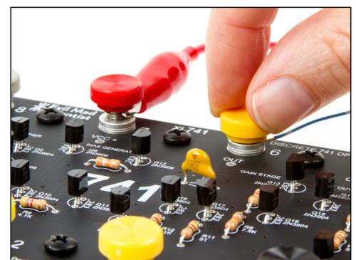
You can connect to the 741 through bare wire, alligator clips, or spade or ring lugs, using the terminal posts. You can also directly solder wires to the small pins next to each terminal post, if you’re careful to clip the wires such that they don’t touch the aluminum legs.
