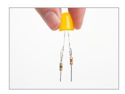
Repeat the procedure, twisting the remaining zero-ohm resistor to the long lead of the LED. Check that the height of your LED with its extended legs is taller than your lower LEDs. If needed, clip the lower wire ends to at least 0.3" below the resistor and jumper, so that you can insert it into the breadboard. Install it to the breadboard with the resistor at row 31, blue stripe, and the zero-ohm jumper to Row 32, column c.
