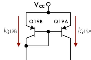
Figure 5: Q19A/Q19B Current Mirror
