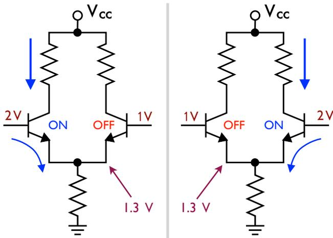
Figure 4: Simplified differential amplifier
