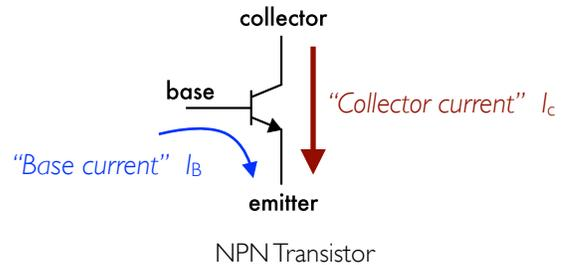
The three terminals of an NPN bipolar transistor are named “base,” “collector,” and “emitter.” The base and emitter pins comprise a diode, indicated by the little arrow on its schematic symbol. A diode is a unidirectional circuit element, so under normal circumstances, current can only be made to flow from the base to the emitter, and not from the emitter to the base.
