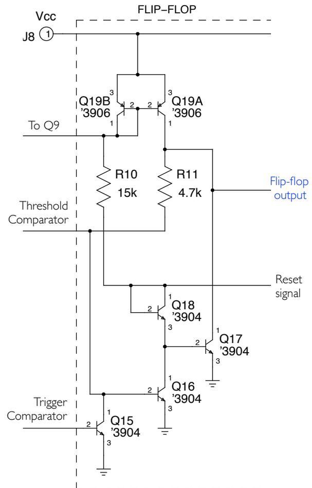
Figure 7: Flip Flop Block
