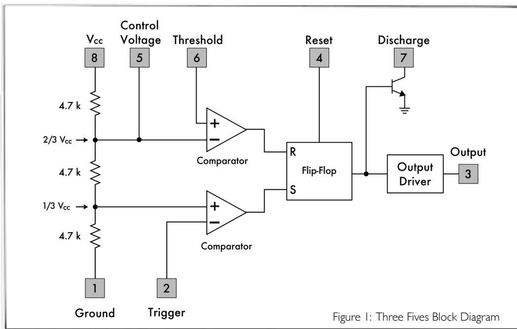
Figure 1: Three Fives Block Diagram
